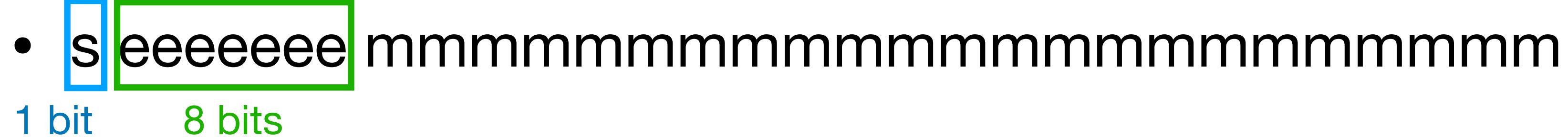
The diagram illustrates the IEEE-754 floating-point format. It shows a sequence of bits: a blue-outlined box labeled "1 bit" containing the "Sign" bit, followed by a green-outlined box labeled "8 bits" containing the "Exponent" bits, and finally the "Mantissa" bits represented by a series of "m"s.
