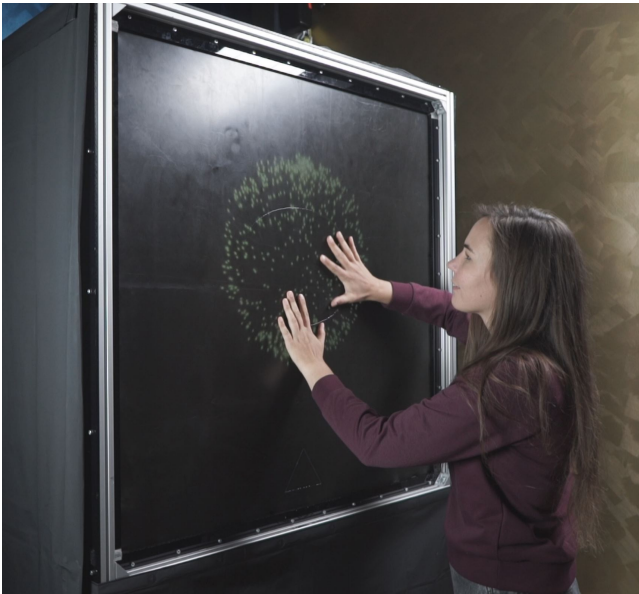
Figure 1: Feeling Fireworks is a large-scale tactile display which generates a tactile firework show, providing an extra dimension for Blind and Low-Vision (BLV) users, in the context of an enjoyable experience that can be shared by BLV and sighted users.
