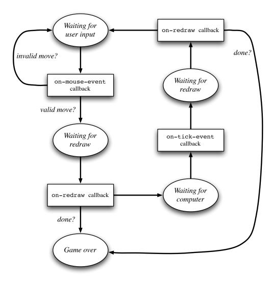
Figure 2: The game states and transitions. The ellipses represent logical states, while the rectangles represent callback functions.
